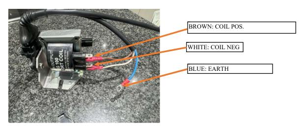
The Module bracket is connected to the coil with double sided tape, this is for transportation. It can be left like this or the tape can be removed.
