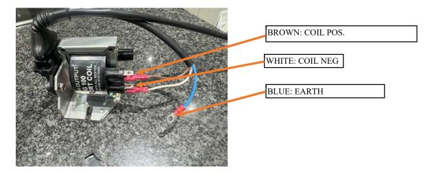
The Module bracket is connected to the coil with double sided tape, this is for transportation. It can be left like this or the tape can be removed.
